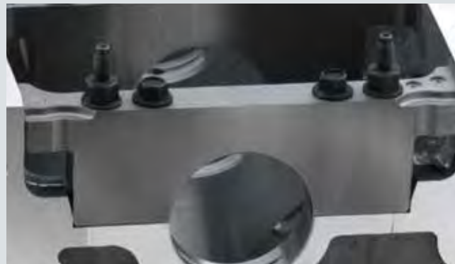
A LS1/LS6 5.7L iron main bearing caps
