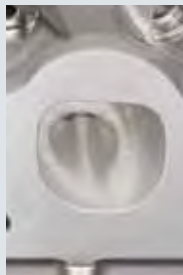
B Close-up shots of the COPO-specific CNC porting applied to a LS7 head. Intake, exhaust and combustion chambers are optimized for COPO drag-race engines
