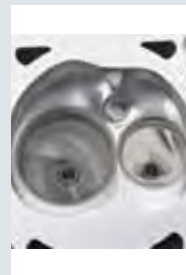
B Close-up shots of the COPO-specific CNC porting applied to a LS7 head. Intake, exhaust and combustion chambers are optimized for COPO drag-race engines
