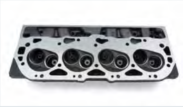
A Bare Cast-iron Gen V and Gen VI Cylinder Head (combustion chamber)
